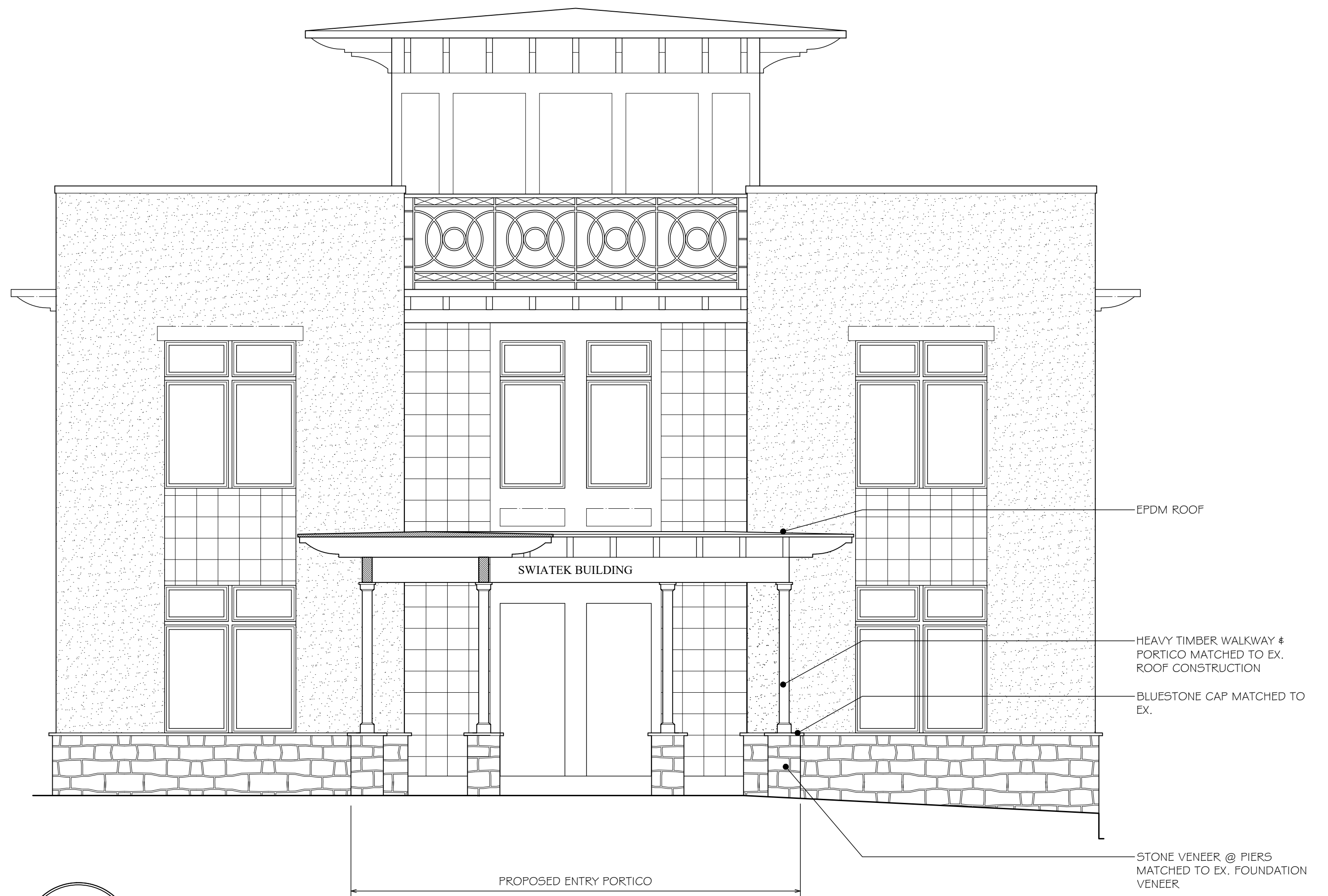
2 SECTION THROUGH BREEZEWAY / NORTH ELEVATION EX. BUILDING 1/4"=1'-0"
